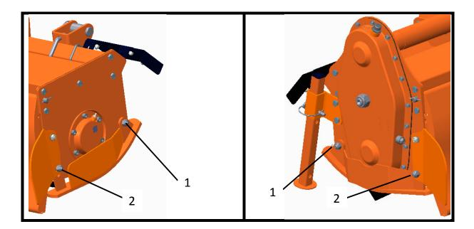
When finished, verify that both skids are at same level, and check if the front of the tiller is leveled to the back, when lowered to the ground. Adjust with the 3-point top link if necessary.
