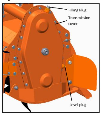
Check the oil level every 50 hours, making sure it reaches the level plug on the transmission cover. If the oil is below this level, fill up oil till restore the level.
