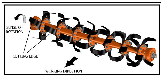
Periodically check the tightness of screws and nuts, and tighten if necessary.
